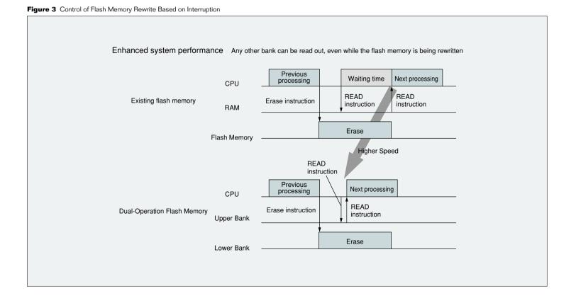
memory-integrated microcontrollers, the interruption can take place in response to any interruption factor generated after the write/erase is completed, thus enabling the processing of other programs after the write/erase command is issued. Write/erase operations for flash memories are smoothly and reliably executed while system control is in progress.
